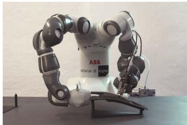
NOWLAB and BigRep developed a robotic additive manufacturing solution to print on existing objects.
